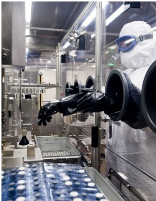
Figure 6B Active RABS (room decontamination)
