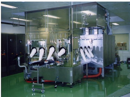
Figure 5B Active RABS (automatically decontaminated)
